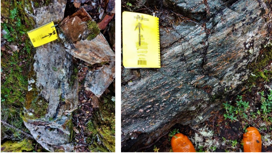
Photo 1A-B: Left - N260 to 280° sheared or laminated rhyolitic tuff with a black quartz vein (sample LC-21-01); Right: Felsic to rhyolitic tuff foliated with pink garnet (LC-21-03)
