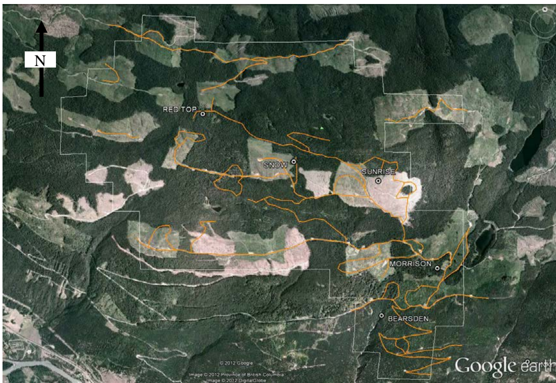
Figure 11. Traverse lines (orange) done by Craig Lynes in 2012 and location of showing (dots) superimposed on a Google Earth image of the Property. White to light grey areas are clearcuts, dark grey areas are forested, black areas are lakes and grey lines are roads. Imagery used by Google Earth is from the Province of British Columbia and is dated 2012.
