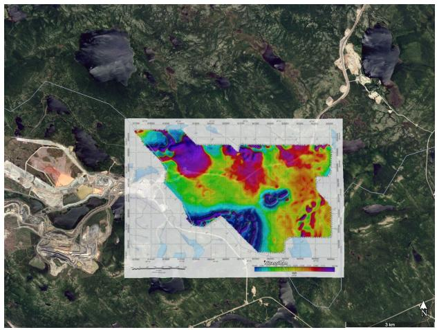
First derivative UAV magnetometer survey image of the main southeast claim block overlain on a recent Google Earth image. Champion Iron Mine's Bloom Lake Minesite and associated mill site are to the left side (west) of the image in the province of Quebec. The bluish purple anomaly in the southwest of the geophysical image is the anticipated iron formation located in Labrador along the Quebec border.
