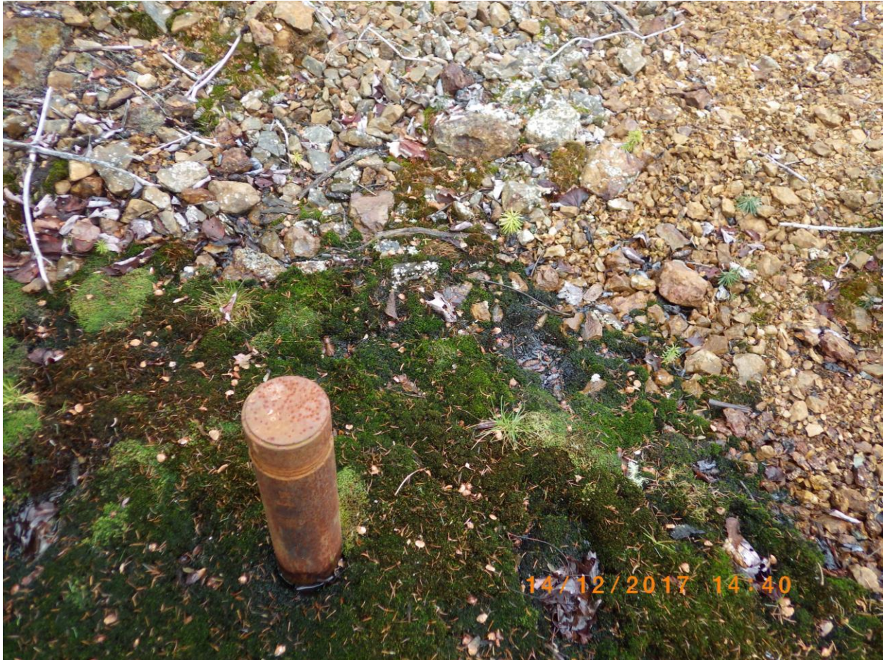
One of several cased & capped diamond drill holes on the Mt Thom Property.
