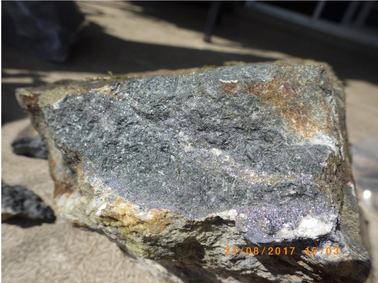
Sample collected from the Galena Pit of the Foster Marshal Property showing subparallel bands of galena and chalcopyrite within Nipissing gabbro.
