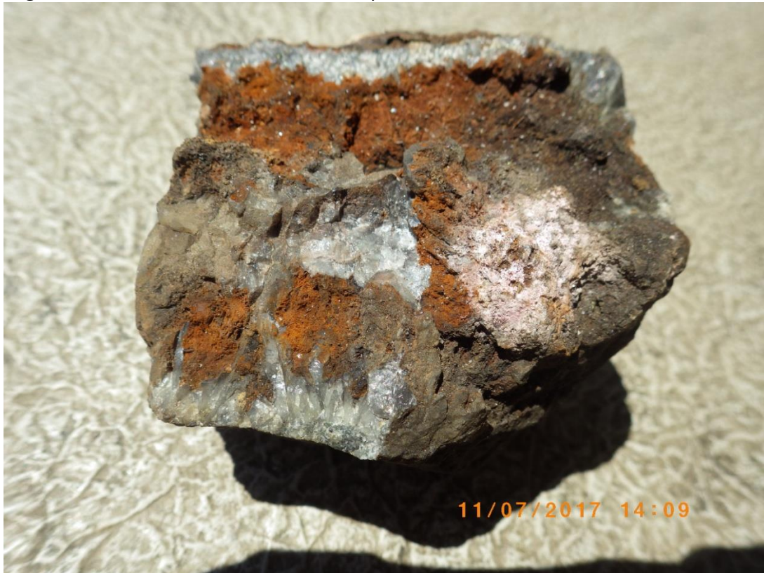
Weathered rock collected from the East Shaft waste rock showing cockscomb quartz, rusty reddish brown iron carbonate and pink erythrite cobalt bloom
