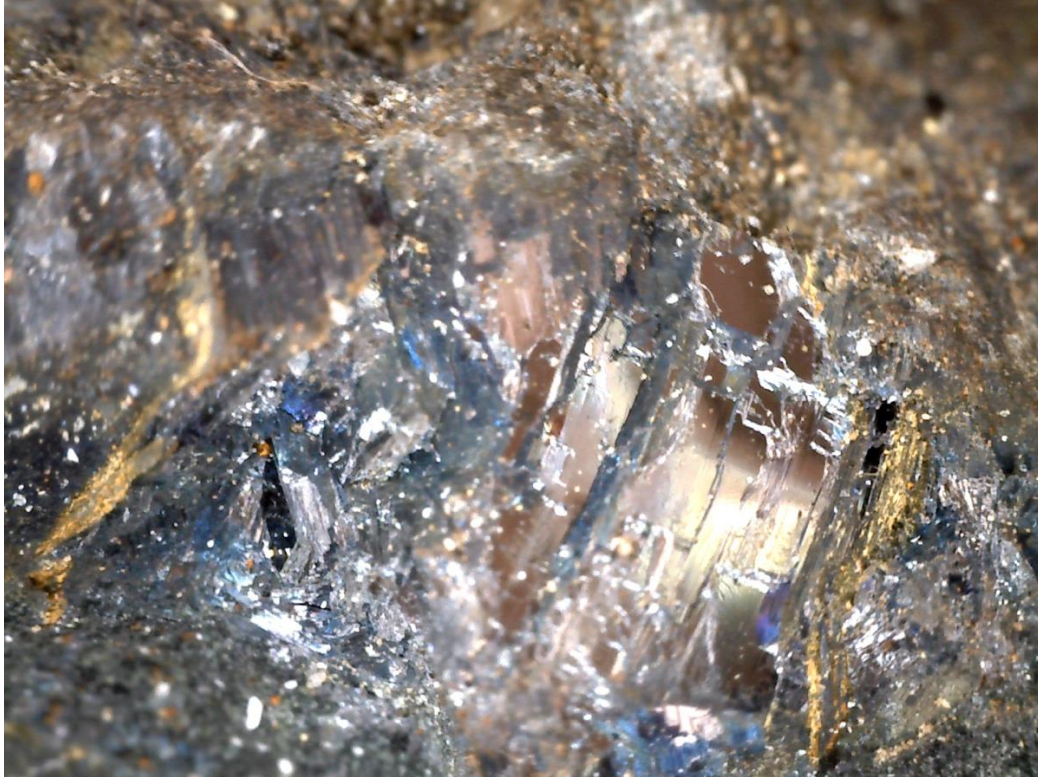
Magnified view of bismuthite from a sample collected from the East shaft waste rock.
