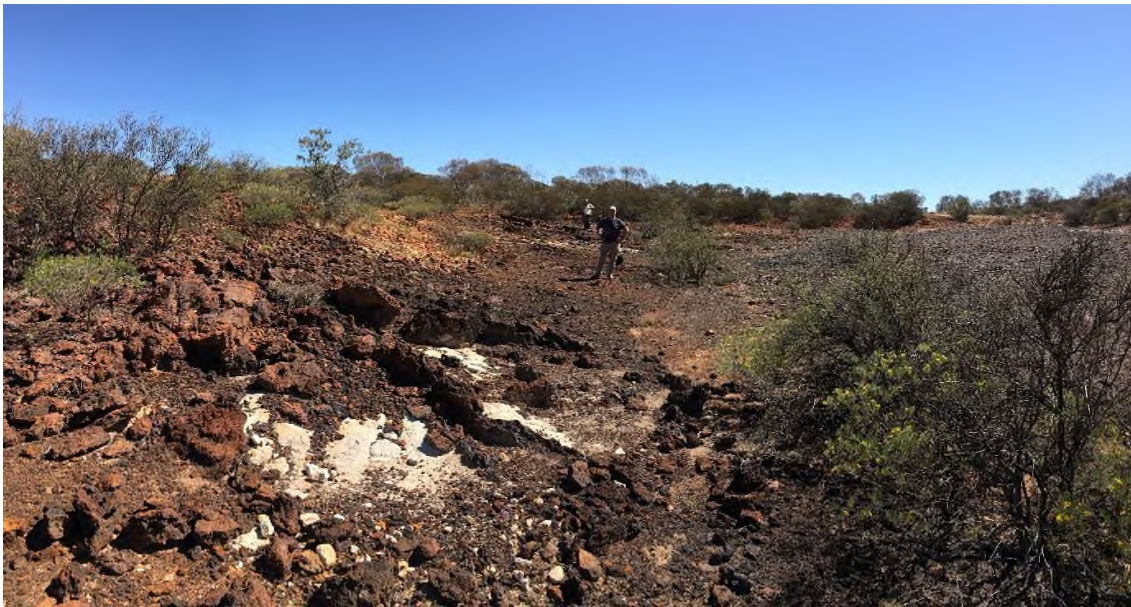
FIGURE 2: Field photograph of highly ferruginous boxwork - textured surface breccia remnant of former sulphide mineralisation.
