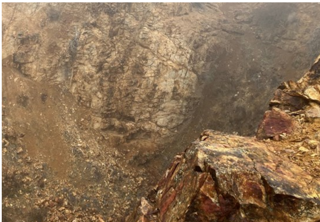
Figure 1 - Historic surface placer mining at Eldorado has exposed parts of the ore zone. The exposed rocks are gold-mineralized.
