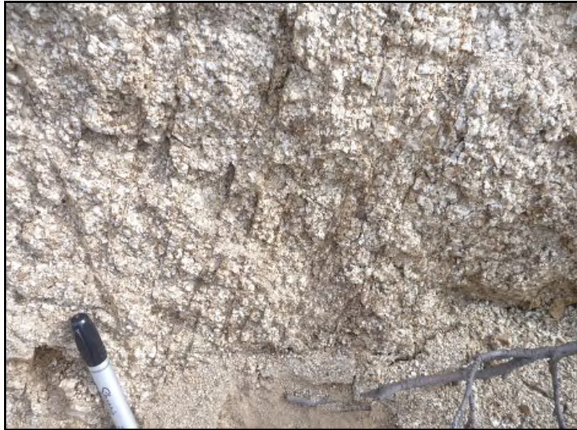
Figure 10: Fine fracture foliation in decrepitated quartz diorite
