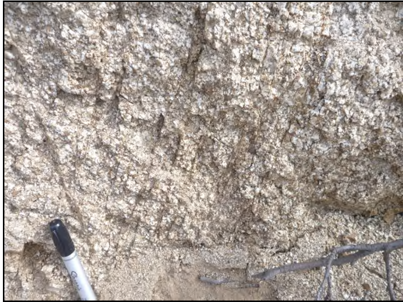
Figure 10: Fine fracture foliation in decrepitated quartz diorite
