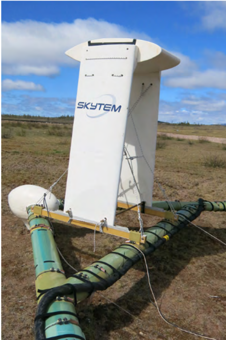
Figure 3 Rudder containing the Z coil located in the top part of the tower.
