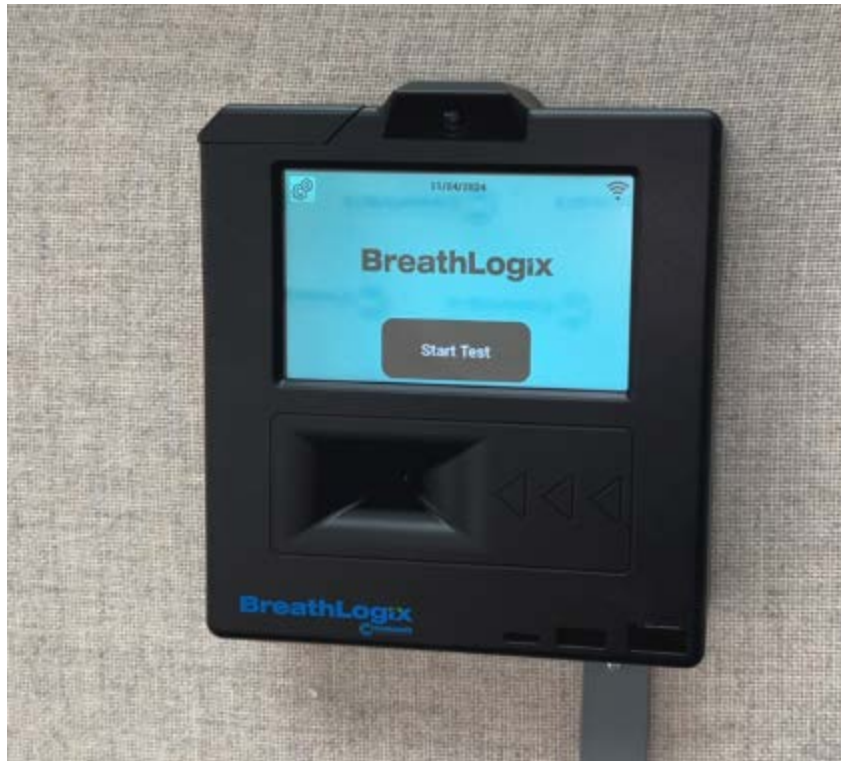
Figure 3. Breath Logix (compact version). Contactless and straw mode both available.
