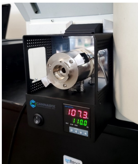
Fig. 4 Cannabix "MS Breath Sampler" technology coupled with Thermo TSQ Ultra
