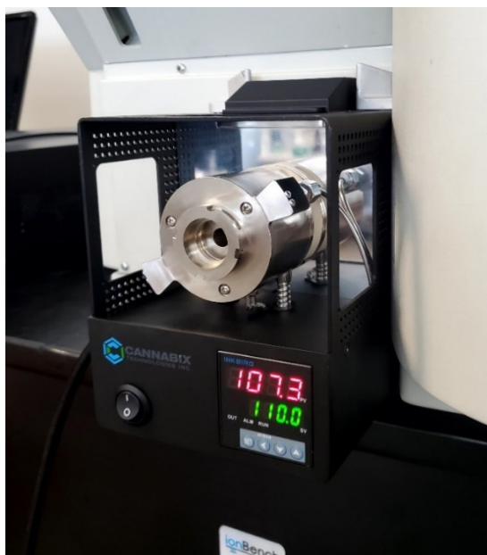
Fig. 1 Cannabix “MS Breath Sampler (MSBS)” technology coupled with Thermo TSQ Ultra
