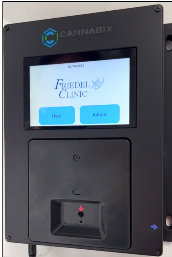
Figure 1. Wall Mounted Contactless Alcohol Breathalyzer Prototype
