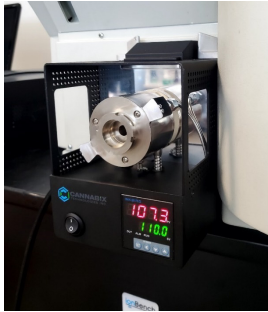
Fig. 2 Cannabix "MS Breath Sampler" technology coupled with Thermo TSQ Ultra
