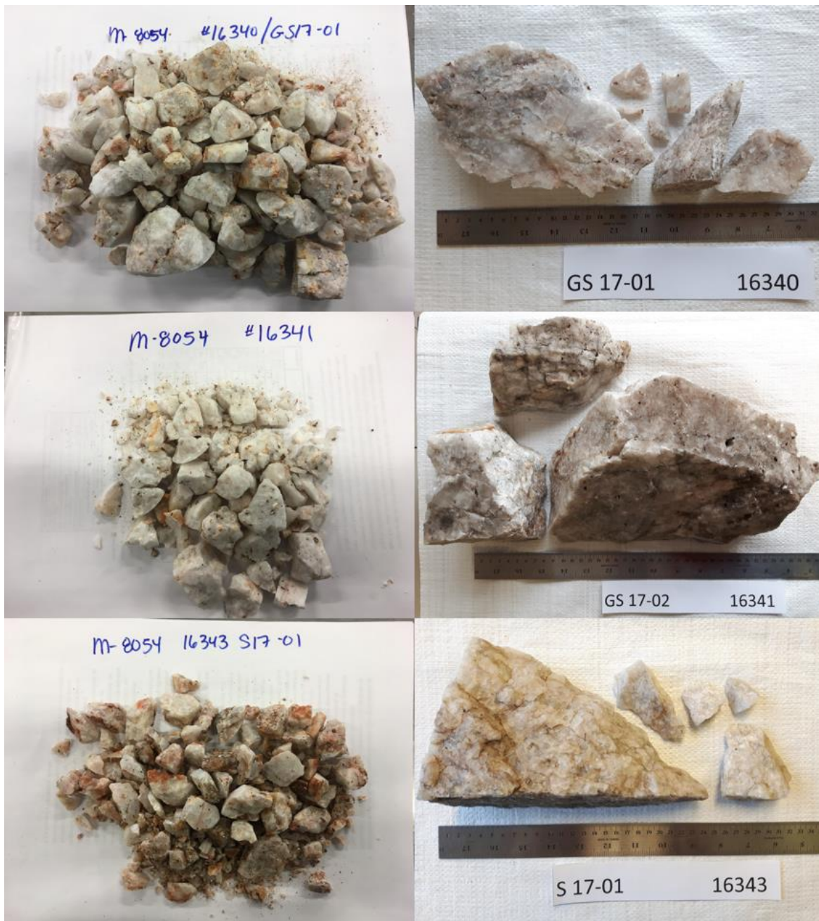
Figure 20: Pictures at the left were taken by CTMP after decrepitation test and to the right were taken before decrepitation test (samples GS 17-01, GS 17-02 and S 17-01)
