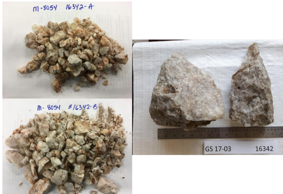
Figure 21: Pictures taken by CTMP before (right) and after (left) decrepitation test
