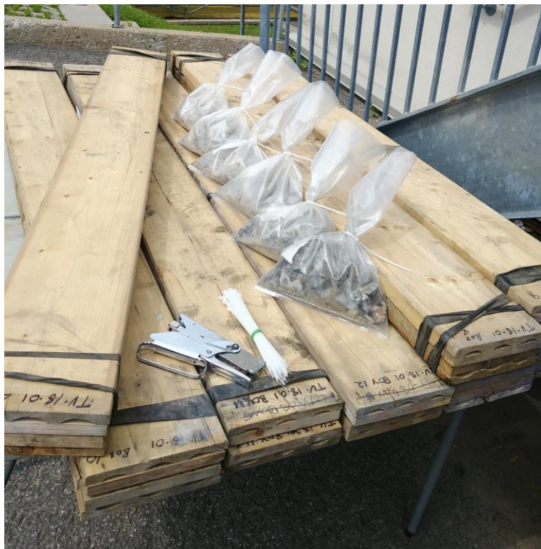
Figure 34. One half of the split core placed in bags and individually tagged; the second half put back in the core box.
