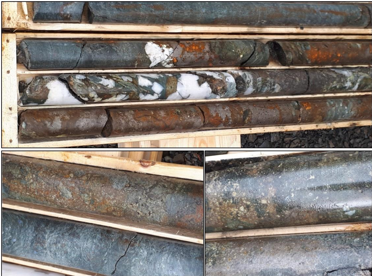
Figure 10: Pictures of drill cores from hole TV-18-018 showing the massive sulphides.
