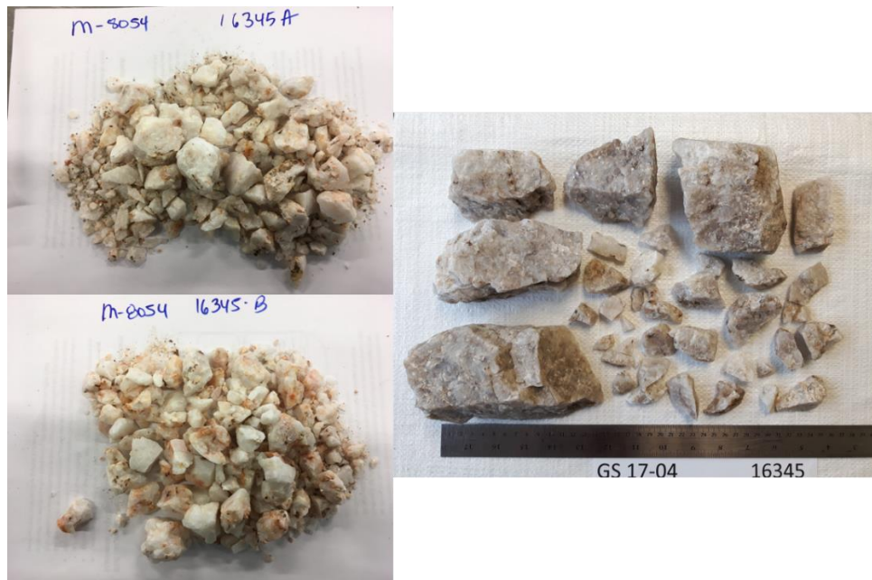
Figure 22: Pictures taken by CTMP before (at the right) and after (left) decrepitation test, (sample GS 17-04)
