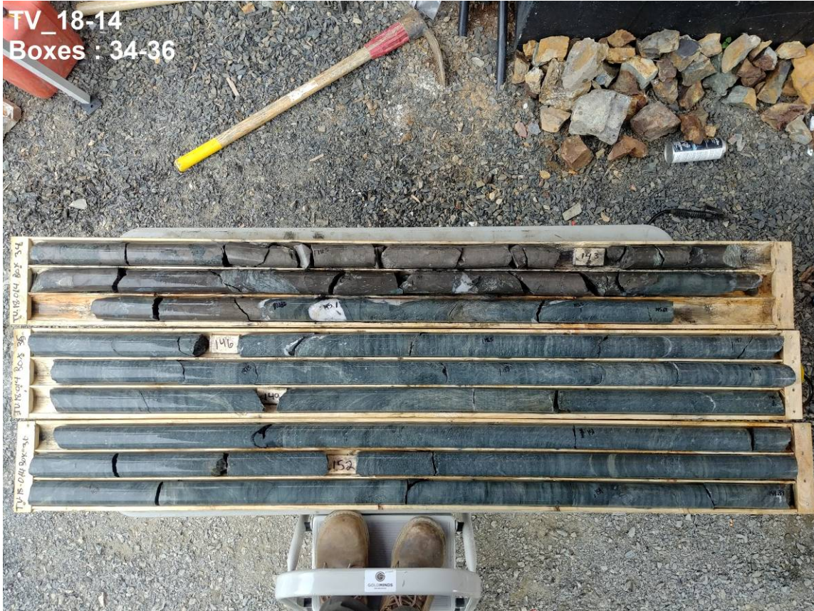
Figure 3: Core split from TV-18-14 at 130m with Chalcopyrite, Sphalerite, Pyrite, Pyrrhotite and Arsenopyrite
