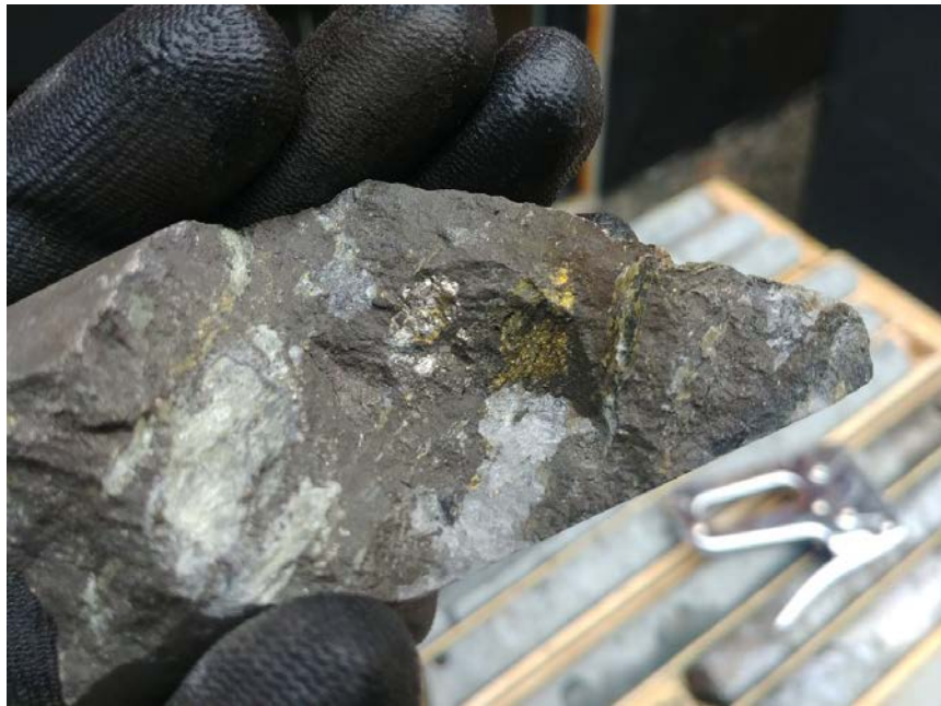
Figure 3: Core split from TV-18-14 at 130m with Chalcopyrite, Sphalerite, Pyrite, Pyrrhotite and Arsenopyrite
