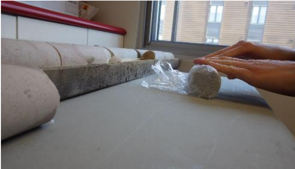
Figure 25: Core wrapped in a Plastic Film to avoid Water Infiltration in Pores
