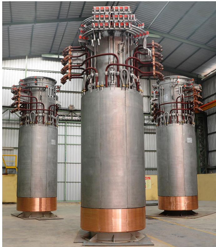
Figure 71: Lower Electrode Columns designed and supplied by Tenova
