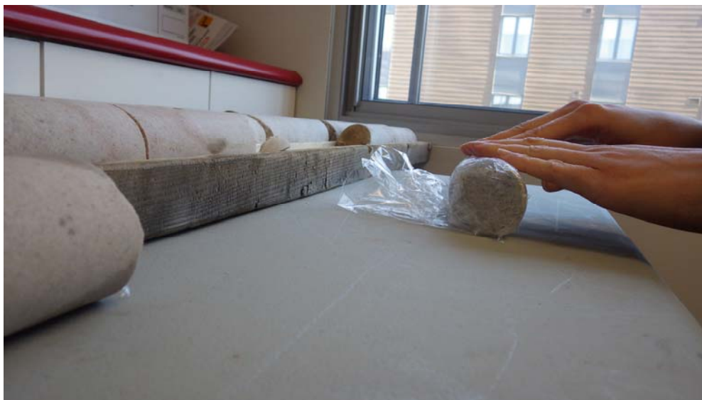
Figure 19. Core wrapped in a plastic film to avoid water infiltration in pores
