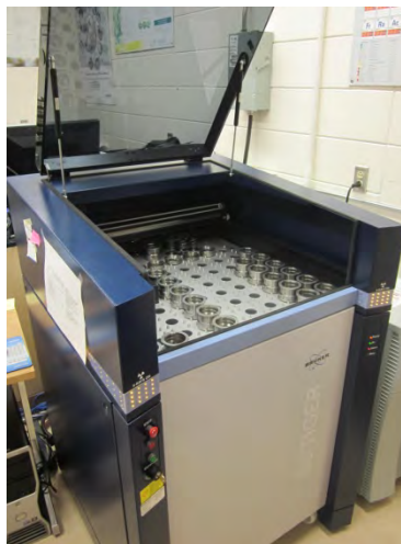
Photo #10 – XRF Bruker S8 Tiger
