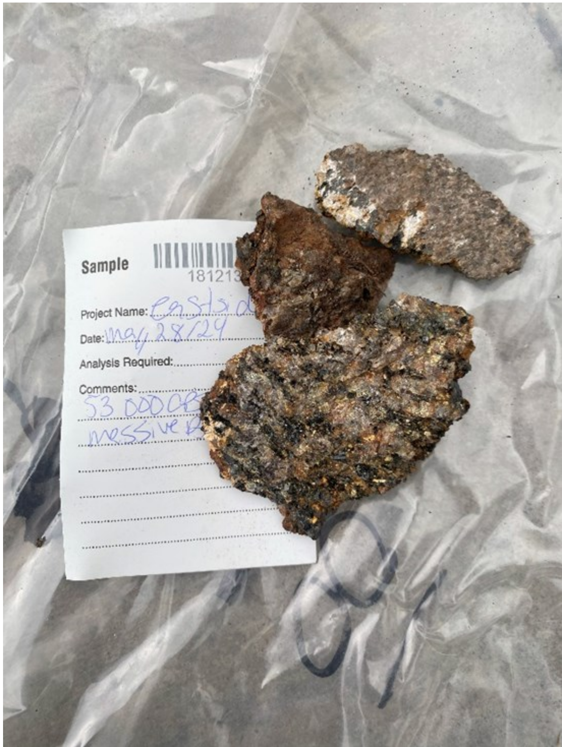
Figure 2 - Uranium sample 181213 displaying 0.25 wt% U 3 O 8 hosted within massive biotite
