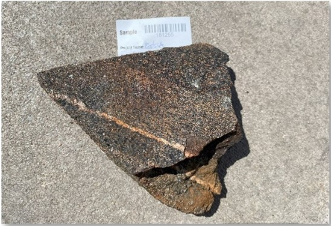
Figure 3 - Uranium sample 181255 displaying 0.07 wt% U 3 O 8 hosted within granodiorite
