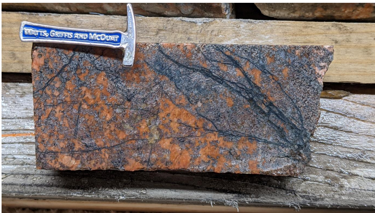
Plate 8: Photo of typical Dante Zone mineralization in DDH DT-19-004B at 16.75 m in sample #0785 - biotite pegmatite with brick red fractured feldspars and strong monazite mineralization with biotite-filled fracturing. Total count radioactivity = 2,700-4,200 cps. (3 cm hammer scale)
