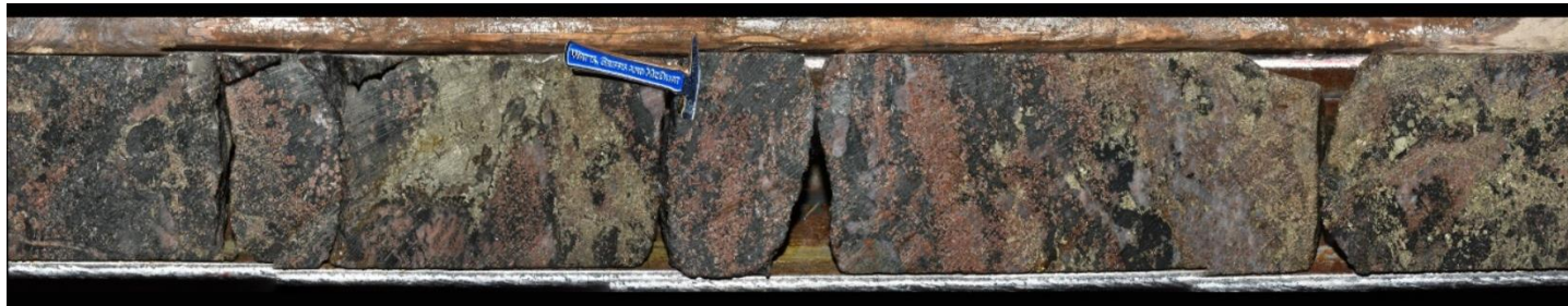
Plate 6: Continuation of above: DDH 21-WRC-016 within section 40.88-41.32 m in sample #2656 assaying 7.34% total rare earth oxides.). Strongly sheared and brecciated zone - pink areas are fine-grained monazite with poikiloblastic pyrite as a void-filling phase. Some original quartz-feldspar boudins. Total count radioactivity = 4,000 to 7,000 cps. (3 cm hammer scale)
