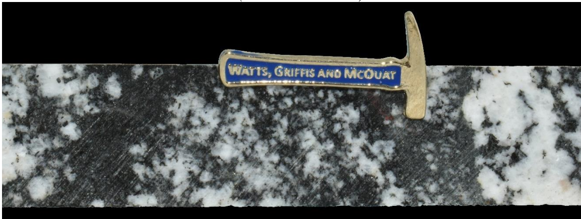
Plate 10: Photo of typical Magnet Ridge Zone: DDH 22-AUG-001: 6.83-7.19 m (sample #003903) - sheared and brecciated paragneiss with biotite. Total count radioactivity = 750-820 cps. 5,200 ppm TREE over 0.36 m. (3 cm hammer scale)
