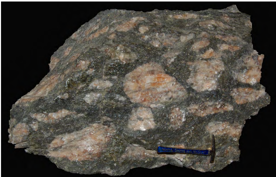
Plate 8: Elliot Lake ore - rounded quartz pebbles in U-bearing, sulphide-rich matrix – 3 cm hammer scale.
