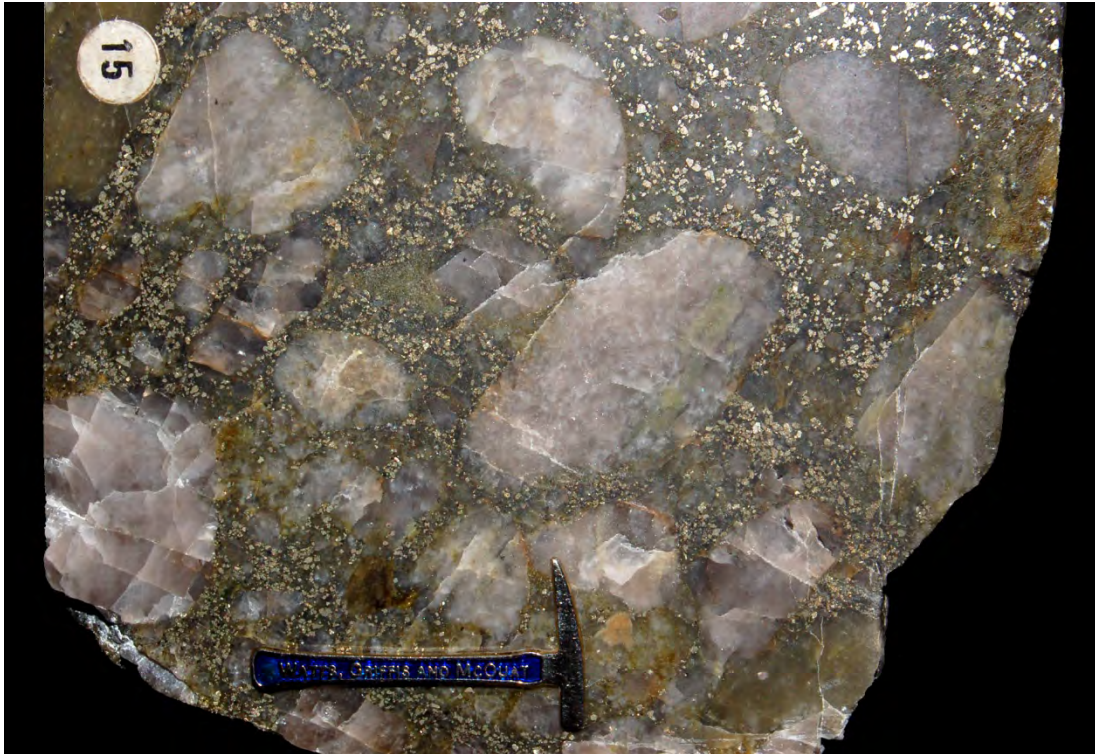
Plate 6: Typical Elliot Lake ore from the Matinenda Formation – compact, well indurated quartz-pebble conglomerate with detrital pyrite and interstitial uranium minerals – 3 cm hammer scale.
