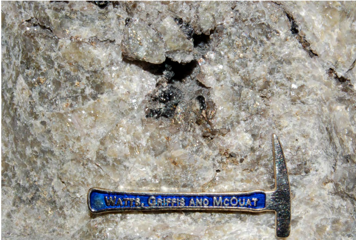
Plate 10: Black thucholite crystals in void in Matinenda Formation quartzite – 3 cm hammer scale.
