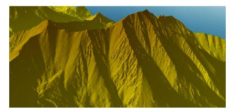
The new 15 cm DEM, down-sampled to 0.5m that was used for the processing of the gravity data. View to the west-northwest over the Beast target (see arrow in map below).
