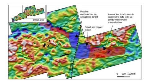
Figure 2. Total counts of radiometrics reveal a zone of lowtotal counts that contains several surface showings in the east part of the property. The zone may continue to the north west as indicated by radiometric, soil, and spectral data.
