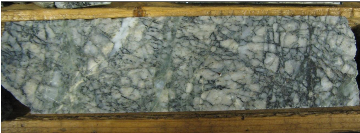
Figure 7.13 Silicified and Brecciated Auriferous LPSE Zone
