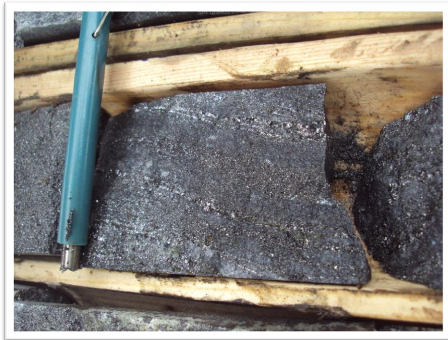
Photo 5: Magnetite-Hematite highly foliated with Specularite parallel to S_0 - S_1
