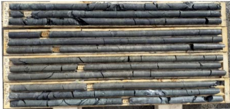
Photograph 1: Massive VMS mineralization from DDH YH22-82 111.8 to 123.0 m in D Zone
