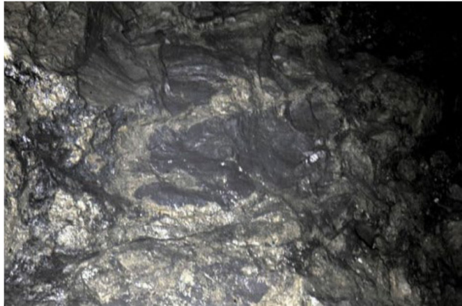
Figure 7-6: Banded and Brecciated Massive Sulfide Mineralization
