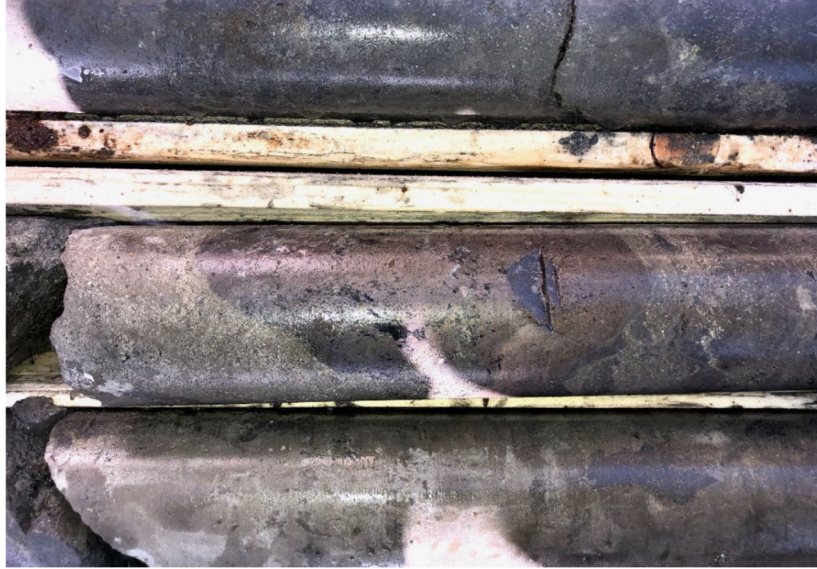
Figure 7-8: Massive Pyrite, Chalcopyrite and Pyrrhotite Mineralization
