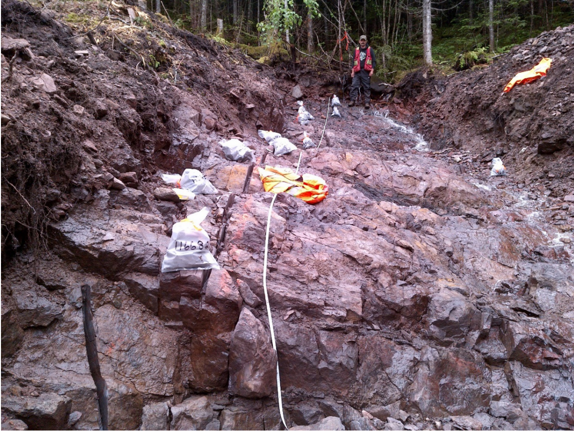
Conducting Channel Sampling Program at York Harbour's Bottom Brook Rare Earth Elements Project, Newfoundland
