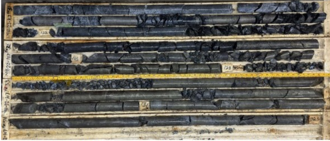
Photograph 2: Massive VMS mineralization from DDH YH22-107 124.1 to 133.1 m in D Zone
