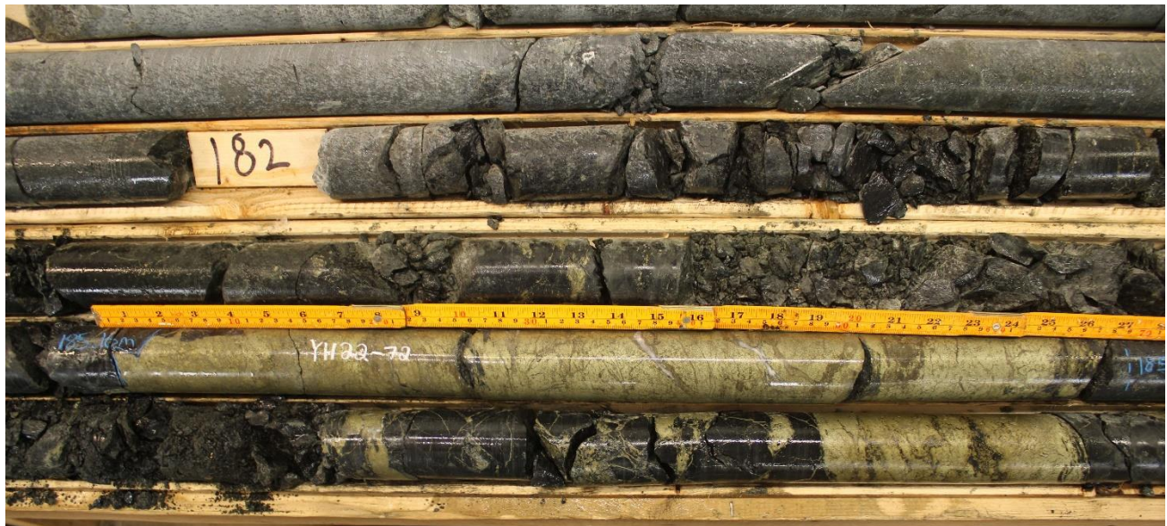
Photograph 1: Massive Chalcopyrite Lens in Drill Hole YH22-72 at 185 m
