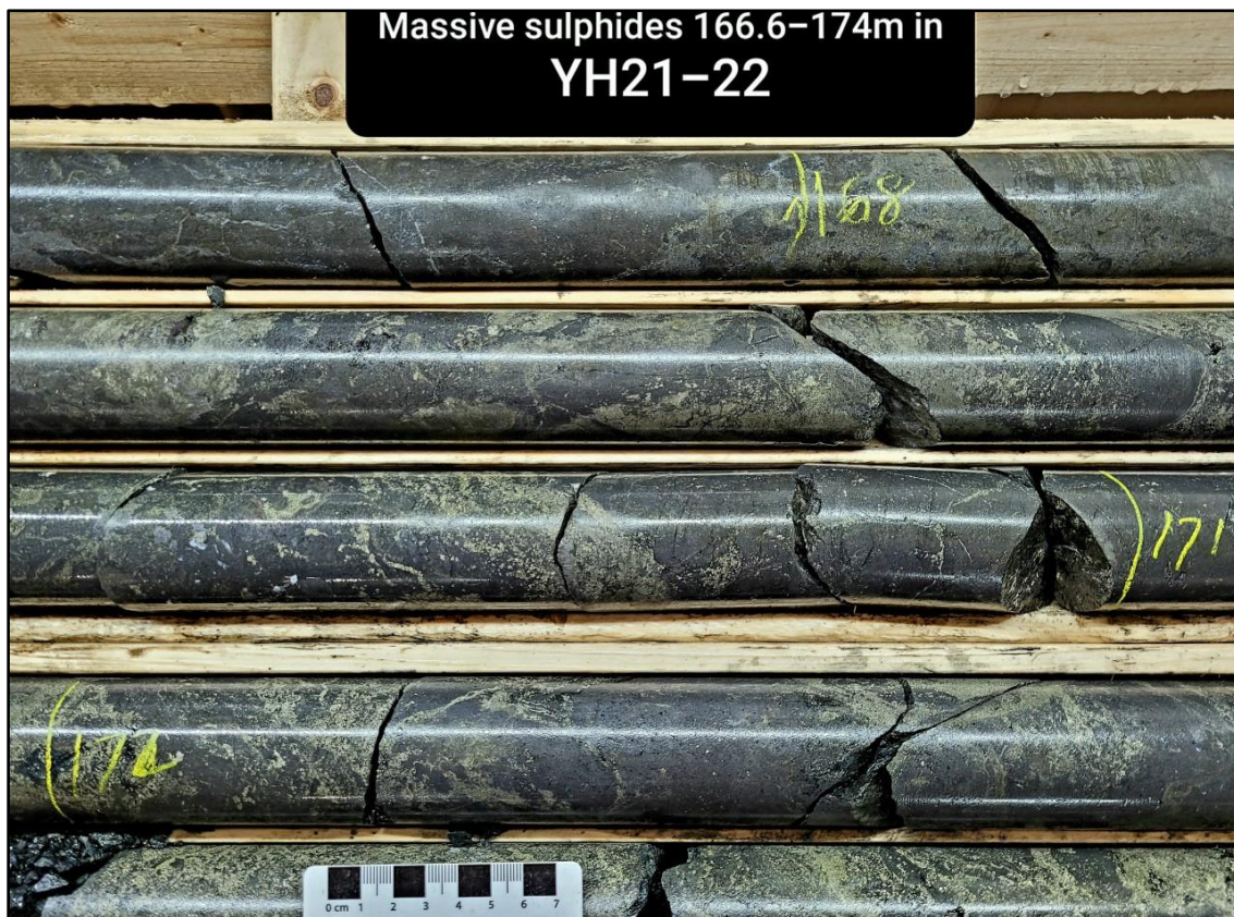
Figure 2: Example of High-Grade Sphalerite (Zinc Sulphide) Intersection in Drill Hole YH21-22 that intersected 5.26 m of 2.84% Copper, 31.96% Zinc, and 42.09 g/t Silver. The dark mineral is Sphalerite.
