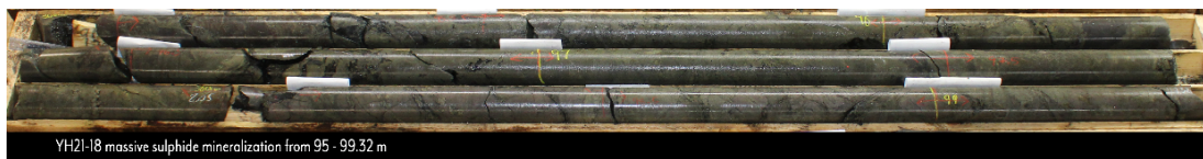
Figure 1: Massive sulphide mineralization in core from 95 to 99.32 metres in DDH YH21-18, part of a longer 25-metre intersection from 93 to 118 metre assaying 2.7% copper, 9.04% zinc, 17.78 g/t silver, 0.15g/t gold and 164 g/t cobalt.
