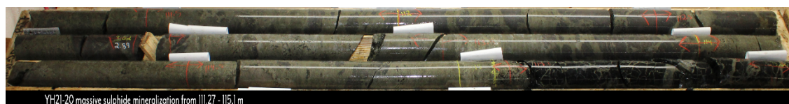
Figure 2: Massive sulphide mineralization in core from 111.27 to 115.1 metre in DDH YH21-20, part of a longer 21.8-metre intersection from 108.4 to 130.2 m. assaying 2.32% copper, 5.94% zinc, 5.17 g/t silver, and 54 g/t cobalt.
