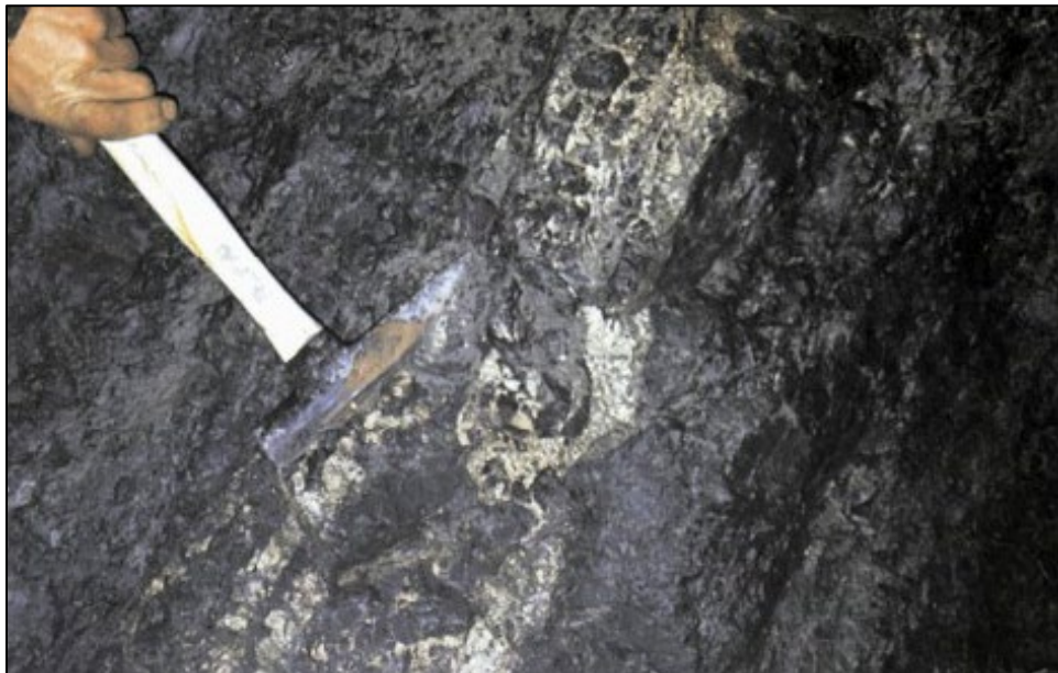
Figure 7-7: Pyrite and Chalcopyrite Stringer Mineralization
