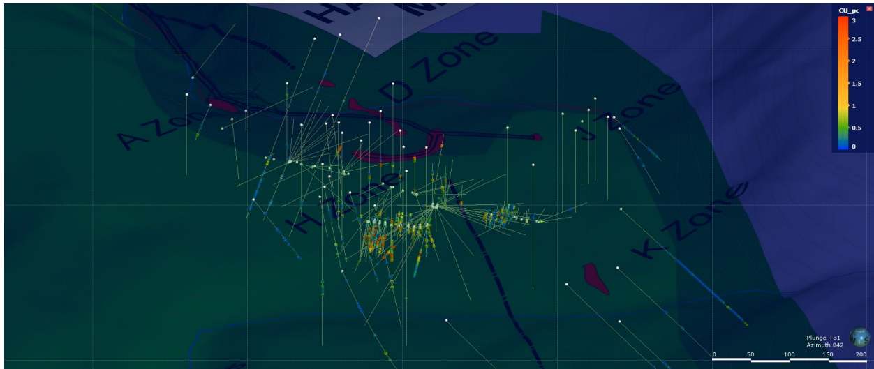
Figure 9-2: 2021 Historical Surface and Underground Drill Hole Traces with Historically Reported Copper Results
