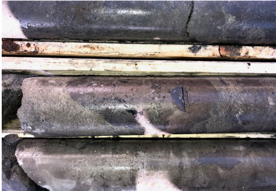
Figure 7-8: Massive Pyrite, Chalcopyrite, Sphalerite and Pyrrhotite Mineralization
