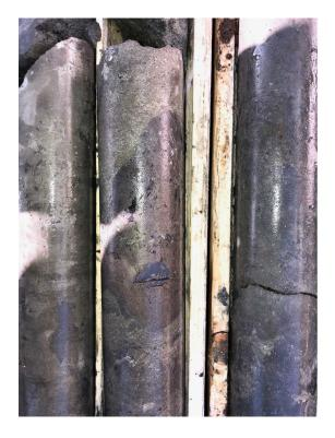
Close-up Photograph of the Massive Sulphide Mineralization in Drill Hole YH21-18
