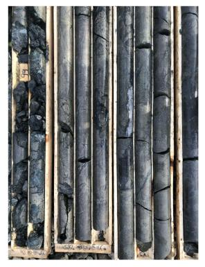
Massive Sulphide from the 10 m Intercept in Drill Hole YH21-19
