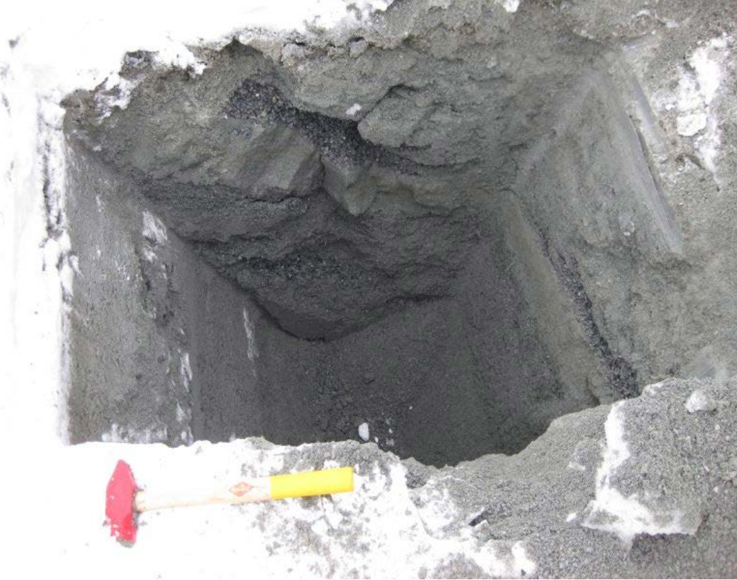
Figure 11.2: Photo of test pit TP19-03. The occurrence of interlayered coarse material was unique to this pit.
