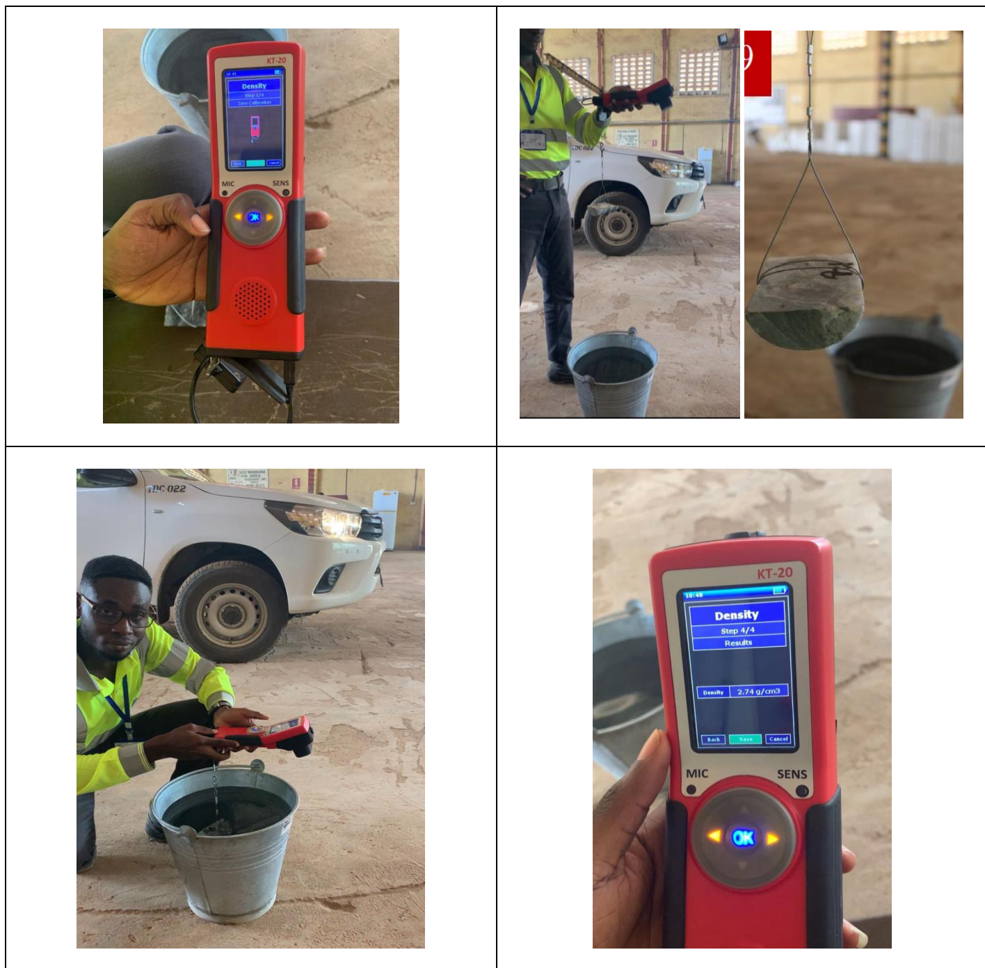
Figure 11-35: Determination of Bulk Density Using Kt-20 (Instantaneous Water Immersion Method)
