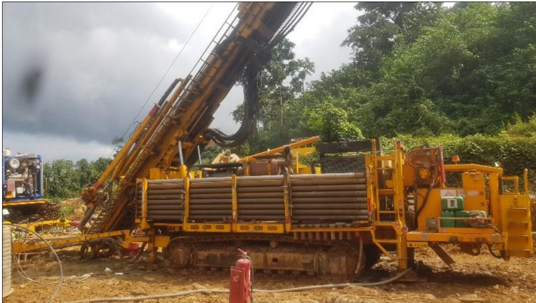
Figure 10-14: Contractor (GeoDrill) Equipment on Aboduabo Project Site
