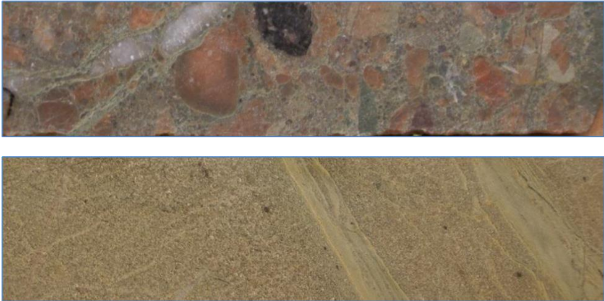
Figure 7-8: (A) Polymictic conglomerate with clasts of granitoid. (B) Tarkwaian arenite sub-arkose
