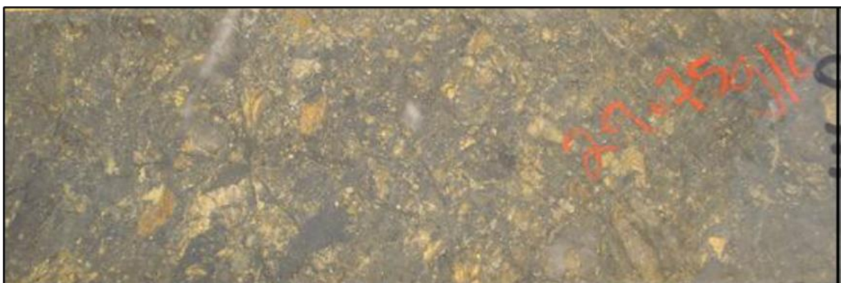
Figure 7-7: Black Breccia at Akwaaba with Gold grade of 29.75g/t
