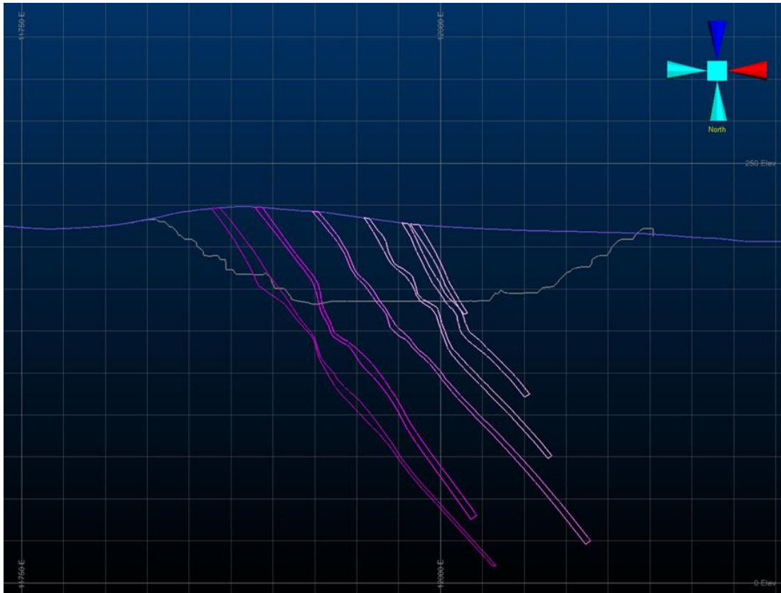
Figure 14-13: Cross Section (6895mn) Through the Strauss Domains Showing Pre-Mining Topography, as Mined Pit Shell and Mineralisation Domains
