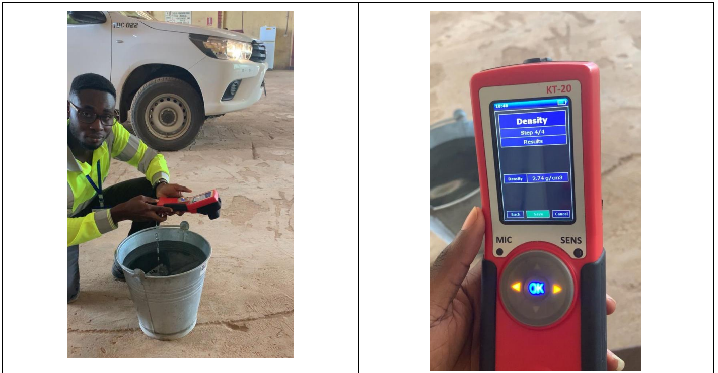
Figure 11-10: Determination of Bulk Density Using Kt-20 (Instantaneous Water Immersion Method)
