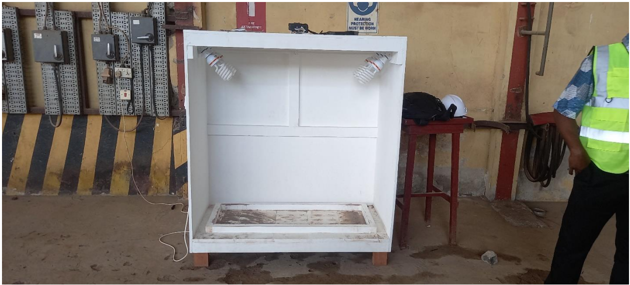
Figure 11-1: Bibiani Project - Core Photography Core Tray Box and Lighting
