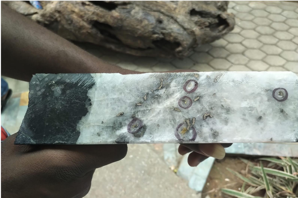
Figure 30: Kubi Main Zone - Photo showing DDHK21-001-89.8m; Garnet Zone/Quartz Vein, Pyrrhotite/Pyrite - Visible Gold in Circles (VG) (true length 24.5cm) (Asante, 2021)
