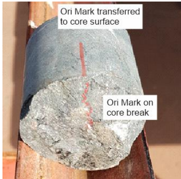
Figure 10.1 Orientation marks on diamond core
