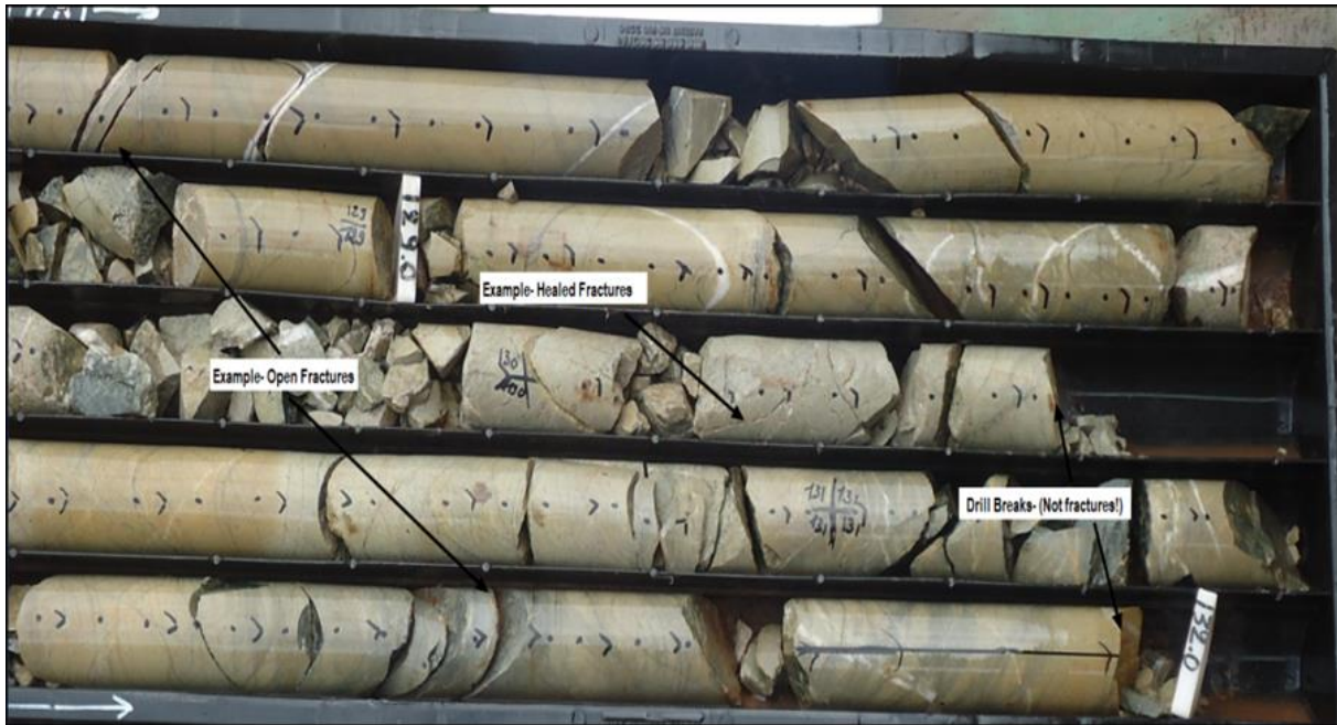
Figure 10.3 Example of diamond core with various degrees of fracturing, and the impact it has on the quality of the orientation mark-up
