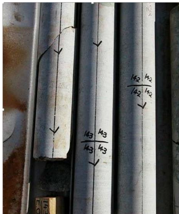
Figure 10.2 Diamond core illustrating the metre mark up, orientation line and down hole arrows
