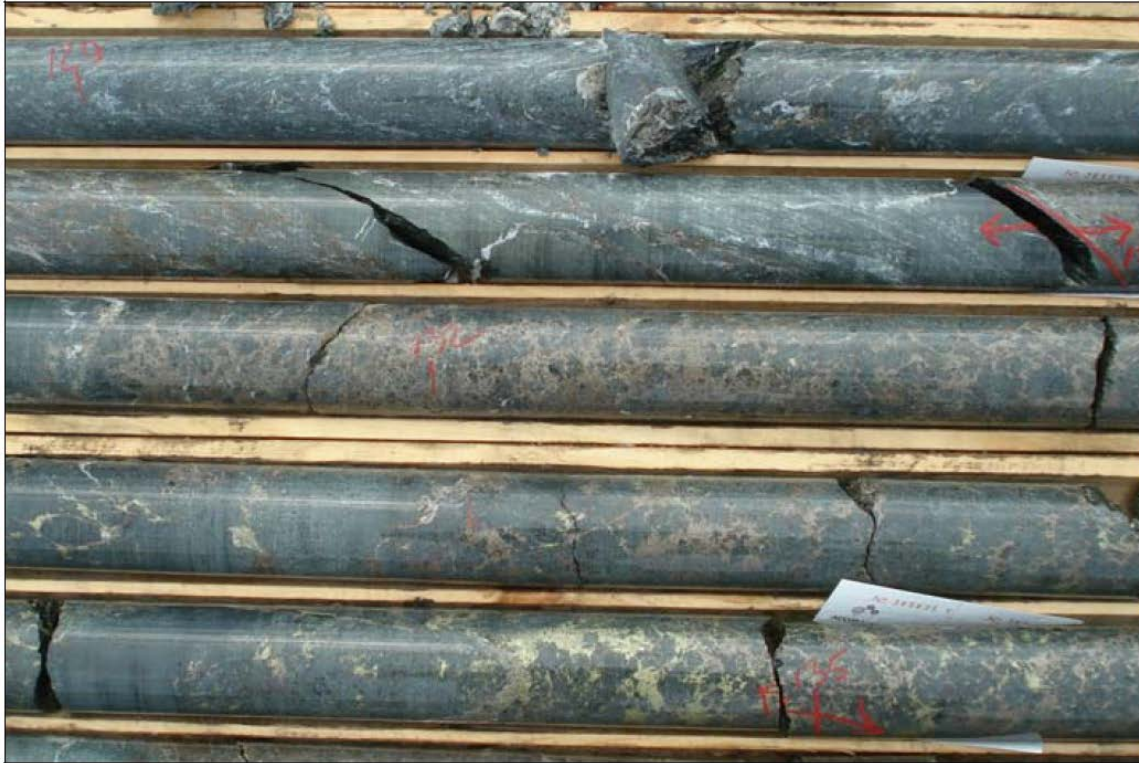
FIGURE 7.8 MASSIVE AND DISSEMINATED NICKEL SULPHIDE MINERALIZATION IN DRILL CORE FROM HOLE K07-119
