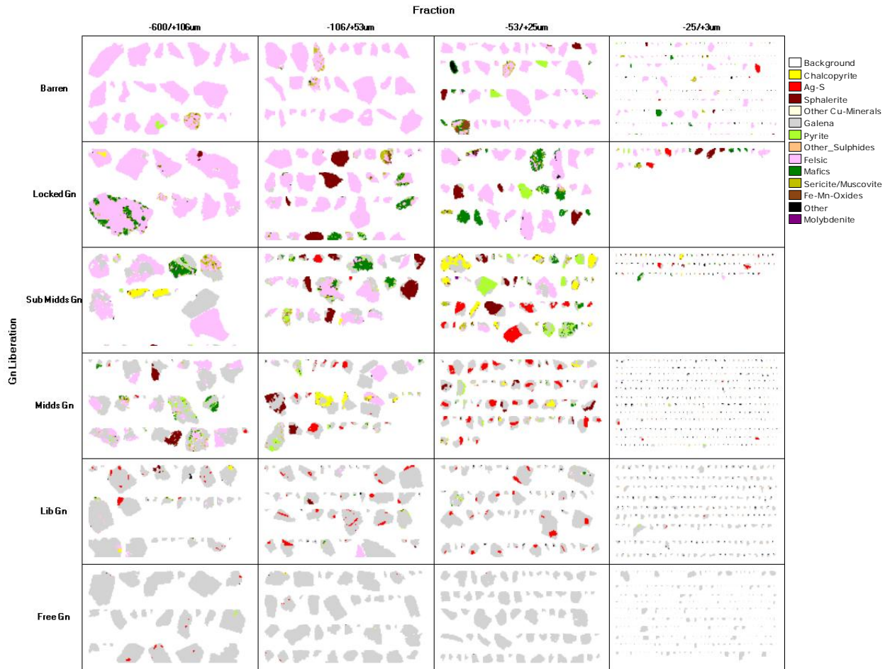
Figure 18. Galena particle maps sorted on the basis of liberation in the sample (PMA)
