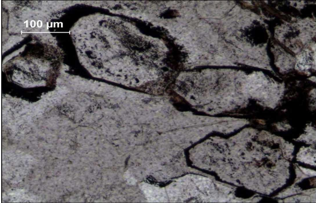
Fig. 15 Sample GR-668-2. Unknown mineral (high-relief, outlined in black), transmitted light, 10x.
