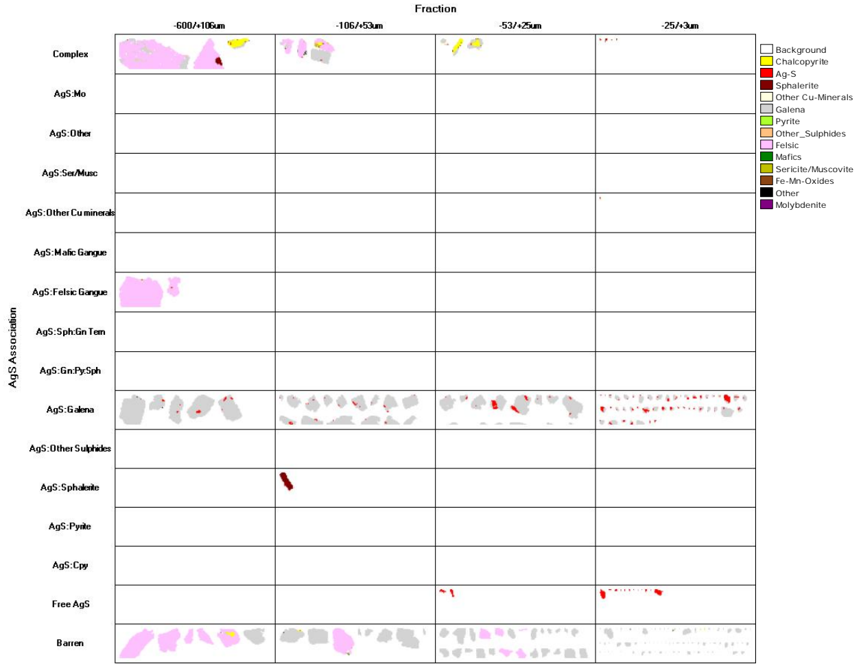
Figure 11. Particle maps of Ag minerals sorted on the basis of association in the sample (PMA)
