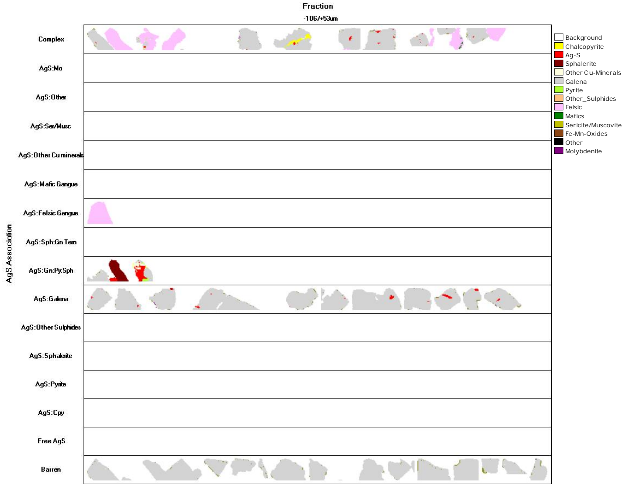
Figure 14. Particle maps of Ag minerals sorted on the basis of association in the 106/+53 um fraction (TMS)
