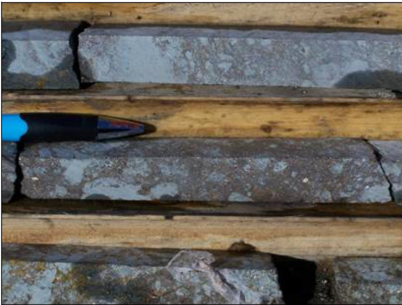
FIGURE 7.9 MASSIVE AND DISSEMINATED NICKEL SULPHIDE MINERALIZATION IN ALTERED GABBRO FROM DRILL HOLE K05-9
