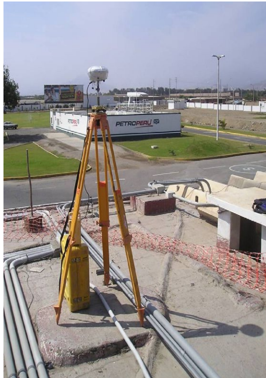
Figure 12.2. A GPS 5800 II measuring the Trujillo airport A-Order benchmark.
