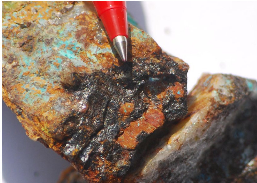
Figure 11.6. Elevated Ag sample containing an anhedral vitreous-luster dark-brown mineral likely causing the Ag anomaly.
