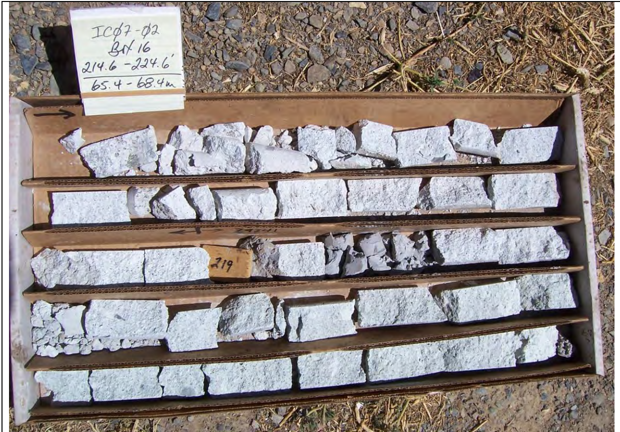
Figure 10.3 – Image of IC-07-02 core from interval 65.4-68.4 m (214.6-224.6 feet); sample 79039 was extracted from 65.23-66.14 m (214.0-217.0 feet). This interval contains 0.187 ppm gold, 1.28 ppm silver, 165.5 ppm arsenic, 23.5 ppm antimony, 10 ppm selenium, 2.44% sulfur, 4.7 ppm tungsten, 5.45 ppm molybdenum and 4 ppb rhenium. The image for Box 15 containing the upper part of the sample interval is unavailable.
