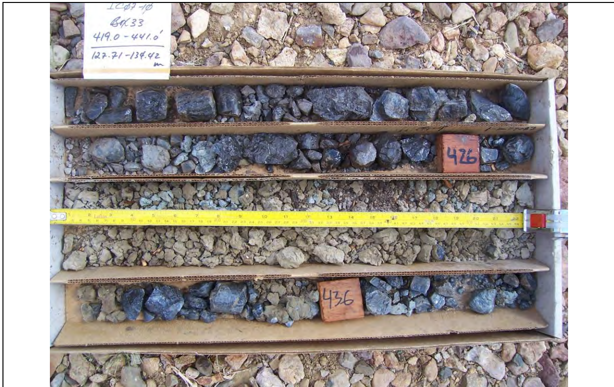
Figure 7.5 – Typical core recovery from interval of high silver values; on average 15%. Core drill hole IC-07-10: 426'-436' (129.9m - 132.9m) returned an assay of 262.0 ppm silver.
